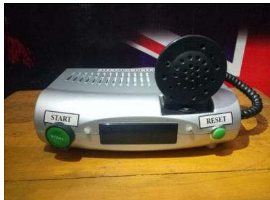
GAMBAR 10 HASIL IMPLEMENTASI ALAT ALCOHOL DETECTOR
